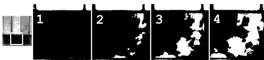
Fig. 8. A sequence of frames from the fluidisation of lactose 16% powder showing a full channel-width powder bed fracture. The area shown in the 4 frames (at times 0.049, 0.050, 0.051 and 0.052s) is the centre of the reservoir, highlighted in the full reservoir image on the left. The images have been converted to binary black and white to improve clarity.
